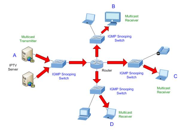
Figure 4-7-5 IGMP Snooping Multicast Stream Control
