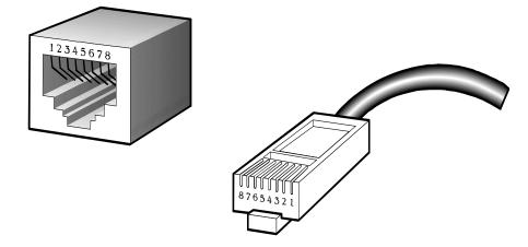
The standard RJ45 receptacle/connector
