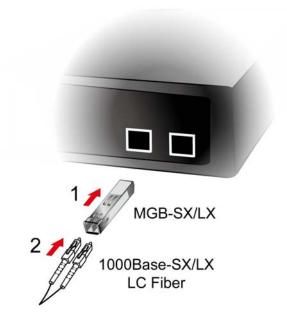
Figure 2-1-7 Plug in the SFP transceiver
