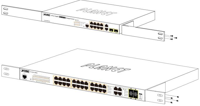
Figure 2-1-5 Attach Brackets to the Managed Switch.
