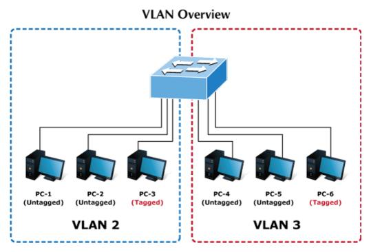
Figure 4-5-20 Two Separate VLAN Diagrams
