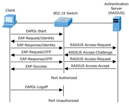
Figure 4-9-2 EAP Message Exchange
