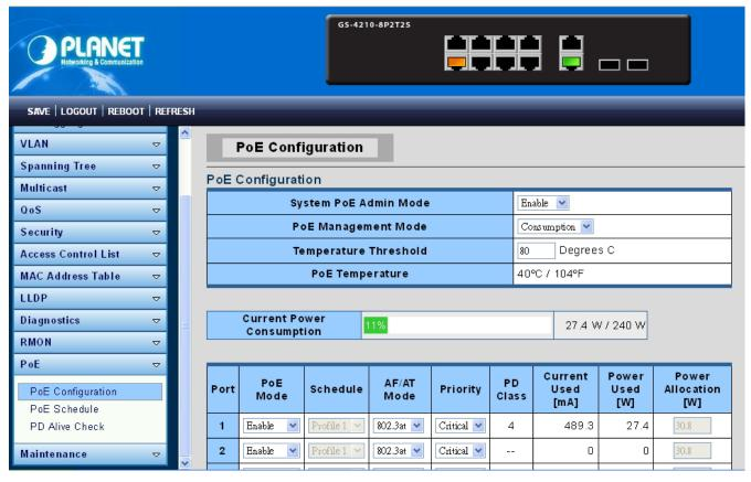
Figure 4-16-1: Power over Ethernet Status
