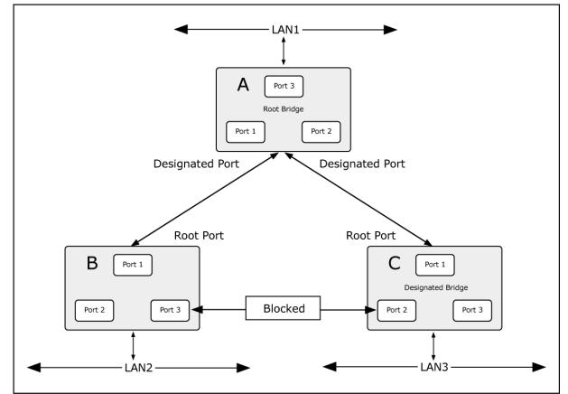
Figure 4-6-3 After Applying the STA Rules
