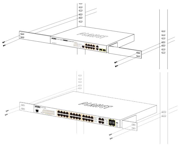
Figure 2-1-6 Mounting Managed Switch in a Rack
