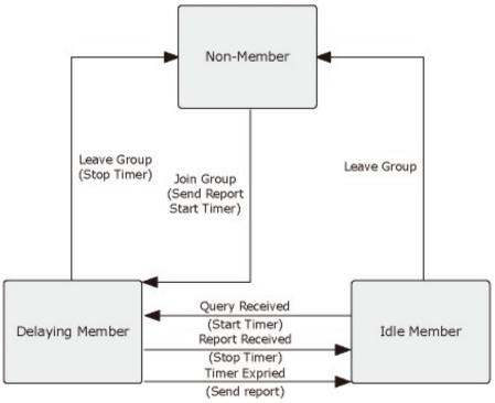
Figure 4-7-6 IGMP State Transitions
