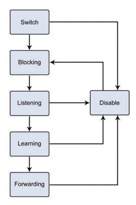
Figure 4-6-1 STP Port State Transitions
