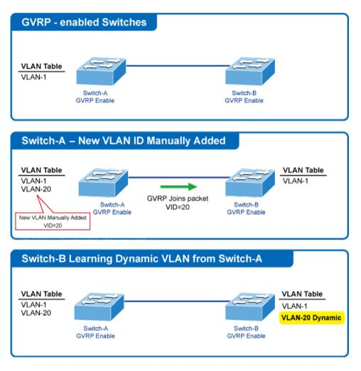
VLANs are **dynamically** configured based on **join messages** issued by host devices and propagated throughout the network. GVRP must be enabled to permit automatic VLAN registration, and to support VLANs which extend beyond the local switch.
