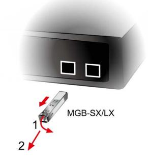
Figure 2-1-8 How to Pull Out the SFP Transceiver
