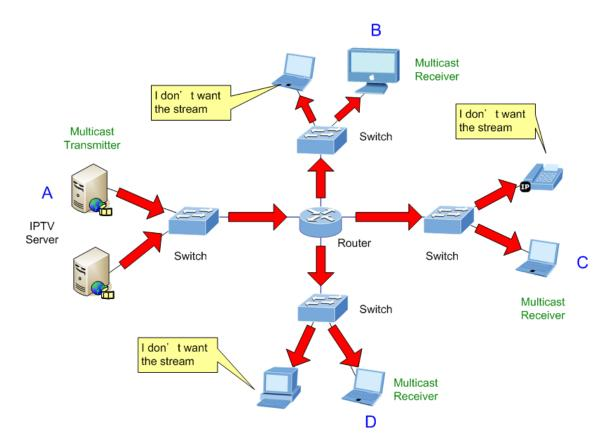
Figure 4-7-4 Multicast Flooding
